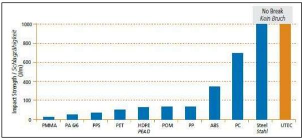
Fig. 3 Notched Izod impact strength [ASTM D256]
