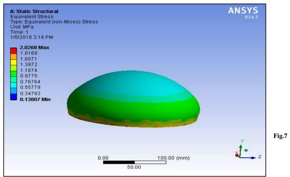
Equivalent stress distribution in Polycarbonate composite prototype.
