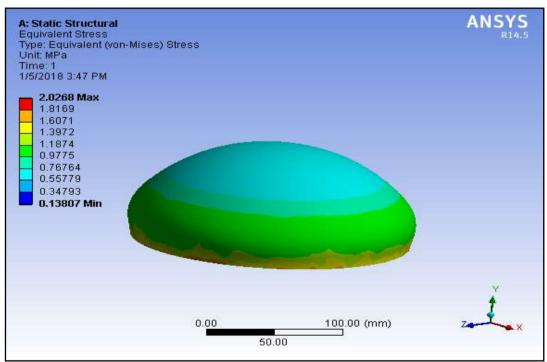
Fig.6. Equivalent stress distribution in HDPE prototype.
