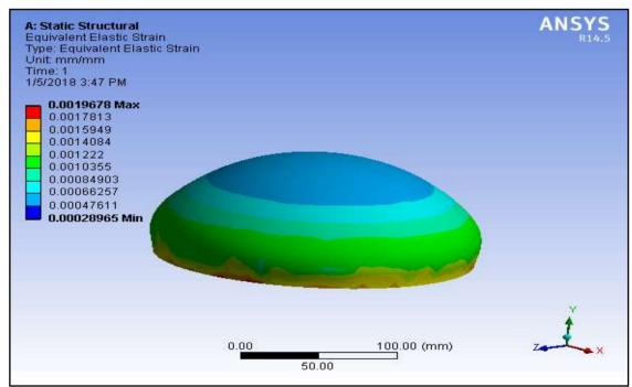
Fig.8. Equivalent elastics strain distribution in HDPE prototype.
