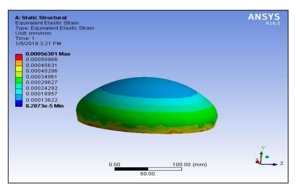
Fig.9 Equivalent elastics strain in Polycarbonate composite prototype.
