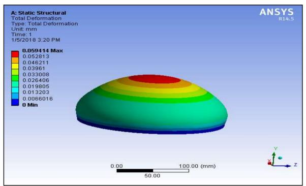
Fig.11. Total distribution in polycarbonate composite prototype.
